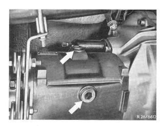
**Take care!** In the case of MB 5-speed transmission, **both** lower drain plugs must be removed when draining old oil, otherwise a large quantity of old oil will be left in the transmission (see adjacent drawing).
