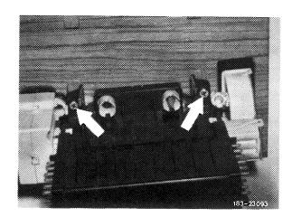
B. Removing and installing temperature dial
