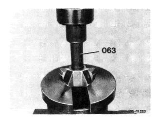
6 Pull stop sleeve and rubber sleeve from rear axle shaft.
