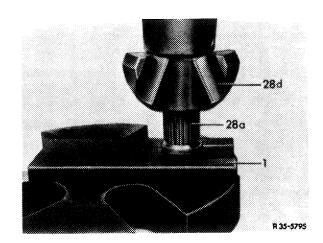
17 Press on spider joint hub (28d) of 2nd version (without stop surface) by means of installing mandrel (063) until mandrel rests against cone of rear axle shaft.
