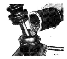
25 Attach rubber sleeve on stop sleeve and on rear axle shaft with new hose clips, while sliding sleeve up to bead machined on rear axle shaft.
