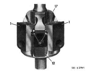
20 Place new sealing rings (13 and 22) on spider (12) and attach new protective sleeve (20).
