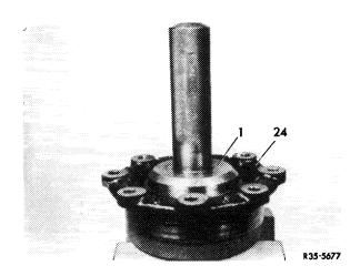
10 Force out bearing outer race by means of removing tool (1).
