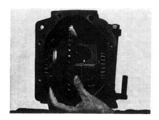
12 Move differential into position shown and take out of rear axle housing (small center piece).
