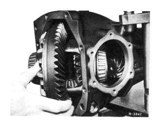
Note: If the wheel assembly is used again, mark position of ring gear in relation to differential housing, so that the ring gear is reinstalled in the same position as before.
