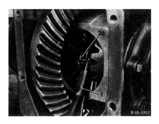
5 Pull rear axle shafts out of side gears and remove together with spacing rings (11).
