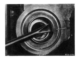
19 Screw installer and remover (1) to rear axle housing and pull inside tapered roller bearing outer race out of housing by means of pulling member (2).
