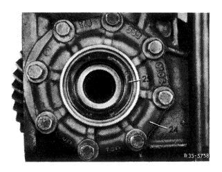
7 Pull off sealing rings (22). Remove compensating washers (23) for adjusting backlash or spread dimension (widening) and mark together with bearing caps (for lefthand and righthand side).
