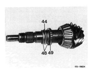
Spacing sleeve Thrust washers Gear wheel (on vehicles with ABS only)
