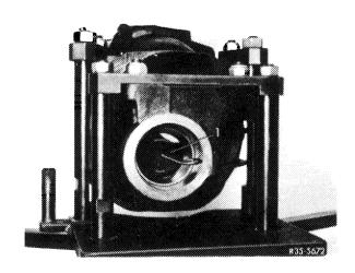
21 Remove spacing sleeve (44) together with thrust washers (48) from drive pinion.
