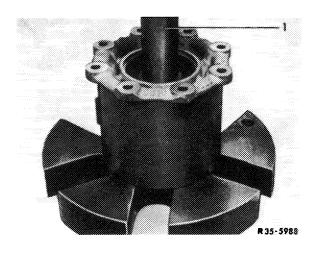
11 Take differential out of rear axle housing (large center piece).
