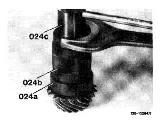
25 Pull tapered roller bearing inner race from drive pinion by means of puller.
