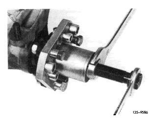
17 Force drive pinion out of rear axle housing by means of a conventional puller.
