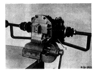
3 Unscrew end cover (4) from rear axle housing.
