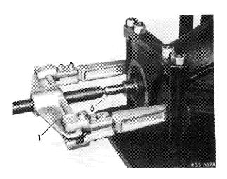
18 Force radial sealing ring (25) out of rear axle housing by means of a screwdriver and remove tapered roller bearing inner race.
