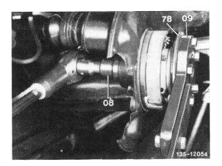
28 Check end play of rear axle shaft flange while moving rear axle flange back and forth and simultaneously turning to the right and left (end play 0.04-0.06 mm).
