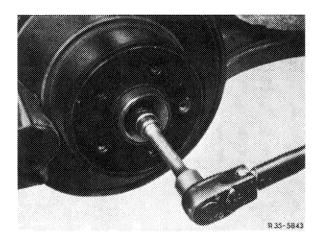
2 If required, push rear axle shaft (28) out of rear axle shaft flange (78) by means of assembly fixture (05).
