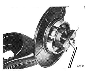
12 Knock bearing outer race of inner tapered roller bearing out of wheel carrier (4) by means of removing mandrel (1).
