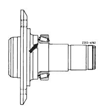
17 For rear axle shaft flange of version used up to now a tapered roller bearing with larger radius may also be used.
