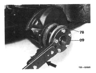
8 Remove sealing race and inner radial sealing ring (6) from wheel carrier by means of a screw driver.
