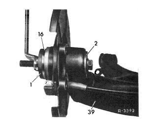
20 Coat seat for outer radial sealing ring on wheel carrier (4) with sealing compound and carefully mount new radial sealing ring (18) by means of puller (1 and 2) so that ring rests against chamfer of wheel carrier.
