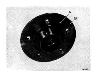
15 If required, refinish oil return spiral with emery cloth (grain 180) at an angle of approx. 20<sup>0</sup> for a length of 25 mm.
