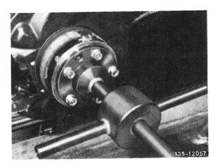
11 Pull bearing outer race of outer tapered roller bearing out of wheel carrier by means of puller (1).
