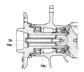
Note: Starting September 1979 the inside contour (arrow) of rear axle shaft flange has been modified and the contact surface of the tensioning washer has been moved inwards by an additional 5 mm. To guarantee the correct association of hex. screw and spacing sleeve, measure distance "a" on rear axle shaft flange from face to contact surface of tensioning washer by means of a depth gauge and take the length for the spacer sleeve and hex. screw from table.
