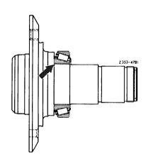
18 Press bearing ring of outer tapered roller bearing (16) on rear axle shaft flange (15) with a matching tube (1)
