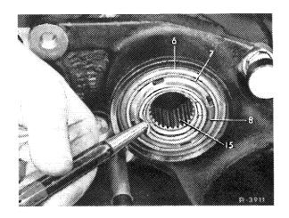
31 Tighten hex bolt for attaching rear axle shaft to rear axle shaft flange of 1st version (M 12) to 95 Nm.
