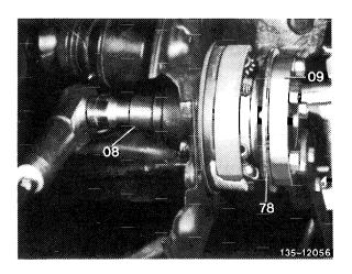
7 With the rear axle installed, the rear axle shaft flange (78) or the assembly plate (09) can be supported with an extension (arrow) as shown in illustration.
