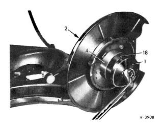
21 Coat or fill both tapered roller bearing inner races and cavity between both bearing outer races in wheel carrier with multi-purpose grease.
