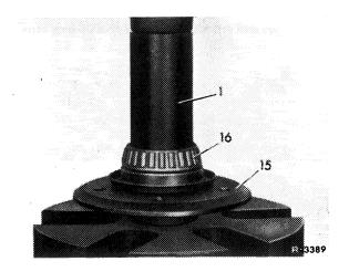
19 Install both bearing outer races into wheel carrier by means of installer (1 and 2).
