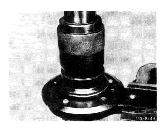
14 Check all parts for re-use. Pay special attention to running surfaces for radial sealing rings on rear axle shaft flange and on sealing ring. Replace worn parts. Check rear axle shaft flange for vertical and lateral runout.
