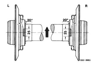
L = Lefthand rear axle shaft flange R = Righthand rear axle shaft flange
