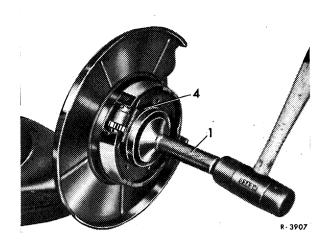
13 Clamp assembly plate with rear axle shaft flange into vise. Pull outer bearing inner race from rear axle shaft flange by means of puller.
