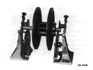
4 If an unbalance if found, drill as many holes on heavy side of new flywheel as required until the flywheels will come to a rest in any position without swinging.
