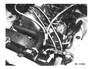
Bleed air-oil cooler prior to measuring consumption.
