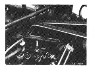
6 Using threaded sleeve, attach dial gauge holder to stud at front right, and to strap for cylinder head cover.
