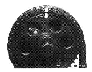
13 Remove camshaft sprocket.
