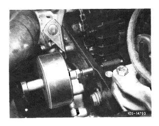
12 Mark positions of camshaft sprocket and timing chain to show how they fit together.
