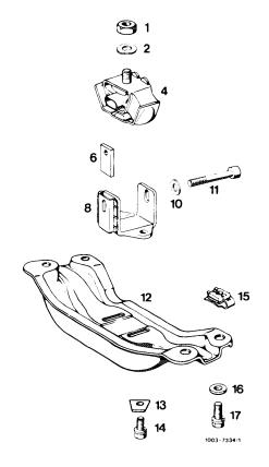
Rear engine mount with stop in models with automatic transmissions
