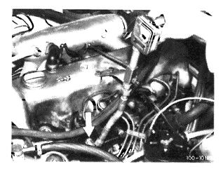
Compression pressure recorder connected to glow plug hole.
