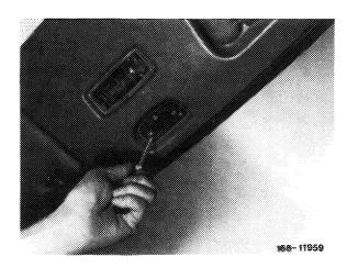
3 Press out roof lamp using a plastic wedge in the opening and disconnect plugs.
