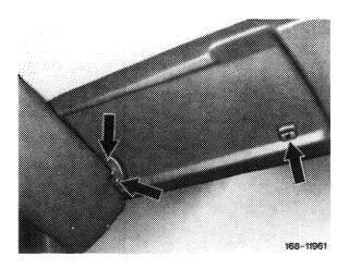
**Note:** The reveal molding of models with a sun roof is held by a chrome plated rail, which must be unscrewed first.
