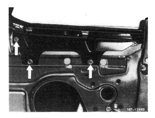
6 Unscrew screw at the front of the box-type column and remove shell cover.
