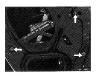
9 Push quarter window down and lift window lifter up and remove.
