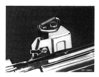
7 Remove lock at intermediate lever of window lifter and disconnect intermediate lever at the guide plate.
