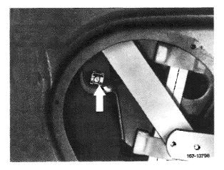
5 Remove screws from window lifter and remove window lifter from the shell via the access opening.
