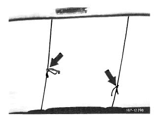
15 Apply light pressure against back window, while at the same time a helper on inside of car lifts sealing lip of rubber frame over spot welded flange of window opening by pulling out the cord, starting at the bottom.
