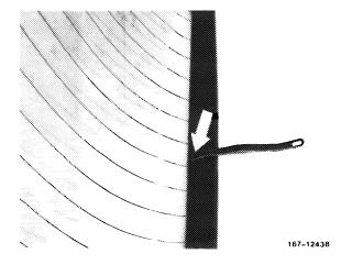
5 Disconnect electric wires at connector on left and right rear pillars.
