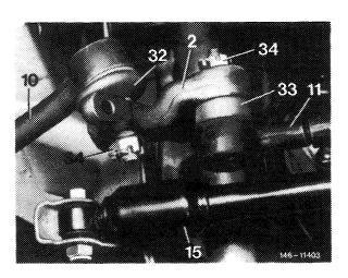
4 Force ball joint of track rod (10) from pitman arm by means of puller (065).
