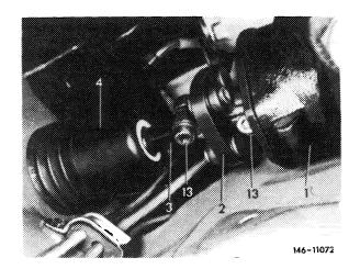
20 Insert pitman arm into splining of steering shaft while watching markings on lever and pitman shaft (arrows).
