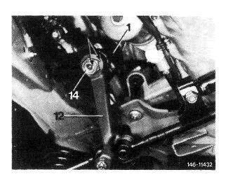
22 Check permissible steering lock by measuring reference dimension between pitman arm and intermediate steering arm and stop bracket of frame cross member (40–320).
