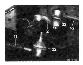
26 Fasten track rod and drag link to pitman arm. Tightening torque 35 Nm — reference value.
