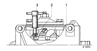
13 Screw center position check screw (060) into steering housing and locate steering nut.
