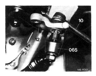
5 Force ball joint of drag link (11) from pitman arm by means of puller (066). On 1st version of drag link, pay attention to plastic covering ring and to sealing washer.
