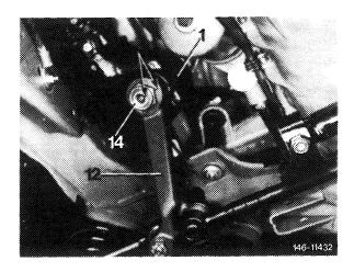
7 Pull pitman arm (12) from pitman shaft with puller (065).
