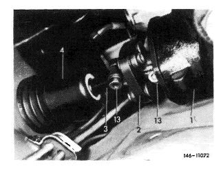
2 Slide steering coupling (2) on profile of lower steering shaft (3) (corrugated tubing) upwards until coupling is no longer in splining of steering worm (1a).
