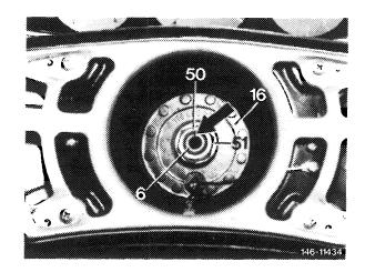
16 Slip steering coupling on splining of steering worm.
