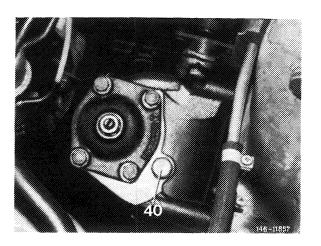
19 Screw both hex socket screws (13) into steering coupling and tighten to 25 Nm.
