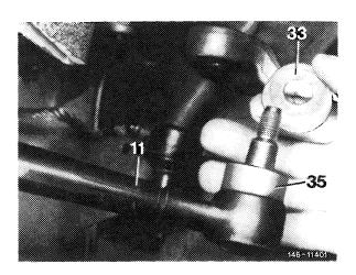
25 On drag link 2nd version, check rubber sleeve (32) on joint. If sleeve is damaged, check joint for wear and replace drag link, if required (46–550).
