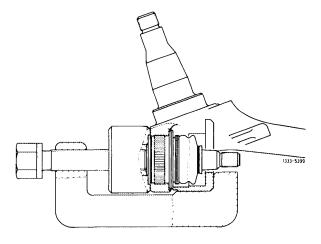
5 Check supporting joint (7) in steering knuckle (5) for correct seat.
