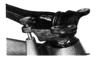
3 Insert measuring indicator into holding device for ball pin of guide joint and move measuring plate into contact with center of measuring indicator.
