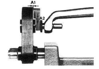
Permissible deformation of steering knuckle in direction of camber (A).
