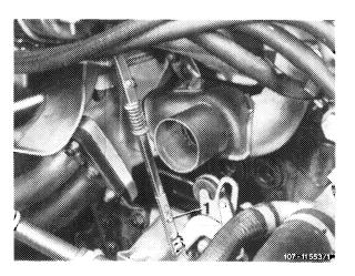
15 Unscrew screw (1) for holder of starter cable assembly and put holder aside, remove grounding cable.
