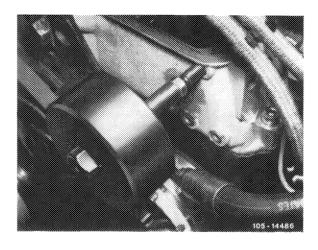
12 Mark camshaft sprocket and timing chain with paint in relation to each other.
