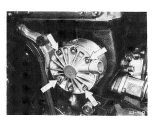
9 On (Aus), (J), (s) and (USA) with power steering starting 1977, unscrew carrier for power steering and air pump. Remove aluminum carrier.
