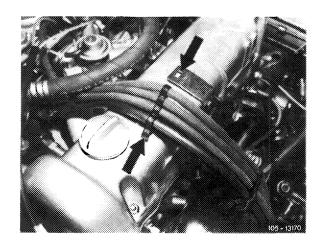
3 On USA 1973—1975, remove vacuum pump with holder.
