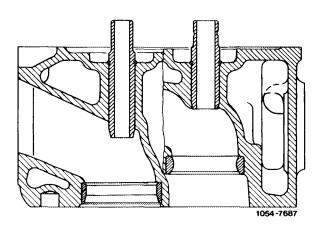
12 Check ID of valve guide with plug gauge.
