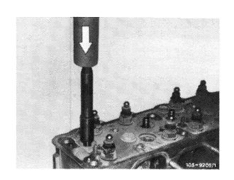
11 Check tight seat of valve guides with cylinder head cooled down only. Tight seat pressure 3500 N.
