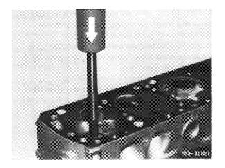
2 Check valve guide basic bore on both bore ends in longitudinal and transverse directions by means of plug gauge.
