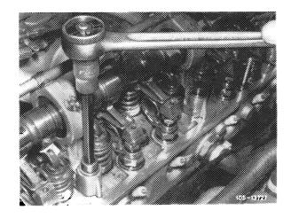
14 Rotate camshaft manually to check for easy operation.
