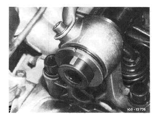
7 Unscrew camshaft bearing bolts with Allen wrench (10 mm).
