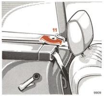
The soft top may become moldy if it is kept enclosed in the storage compartment for an extended period. Unfold and air it thoroughly (do not expose to the sun) at regular intervals during the wet and cold seasons.
