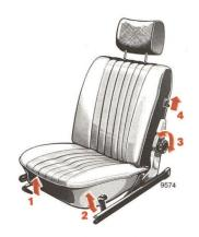
Adjustment of Driver's Seat and Front Passenger's Seat
