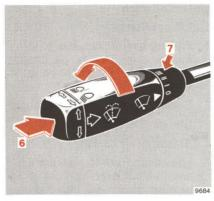
To operate the turn signals, move the combination switch past the point of resistance (up or down). The switch is automatically cancelled when the steering wheel is turned by a large enough angle.
