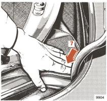
Close top storage compartment cover, making sure that both sides (9) are locked.
