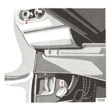
Depress parking brake pedal (1). When the steering lock key is in position "2", the brake warning lamp in the instrument cluster comes on.
