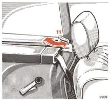
They are used to engage or disengage the locks in windshield header bar and behind the doors (11). Put locking handles back into the glove compartment after use.
