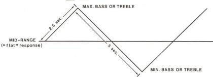
Upon pressing either tone button, the tone level for that function (either bass or treble ) will begin increasing. It stops increasing when the button is released or when the maximum tone level is reached (approx. 2.5 seconds).
