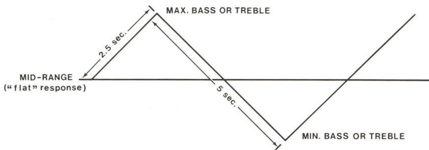
Upon pressing either tone button, the tone level for that function (either bass **[B]** or treble **[T]**) will begin increasing. It stops increasing when the button is released or when the maximum tone level is reached (approx. 2.5 seconds).
