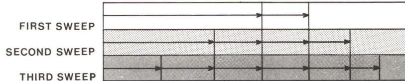
If the station seeker bar is activated within 8 seconds after the radio is tuned to a station, then the search operation will be continued at the same sensitivity level. If 8 seconds are exceeded, the radio will revert to searching only the most powerful stations.
