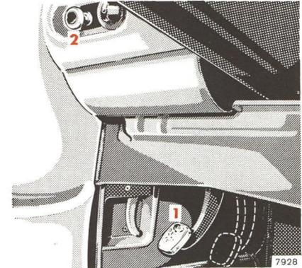
Depress parking brake pedal (1). When the steering lock key is in position “2”, the brake warning lamp in the instrument cluster comes on.
