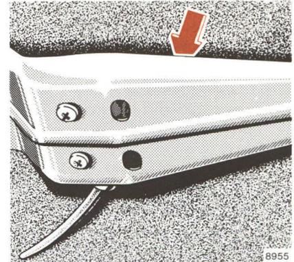
If the central locking system does not release the fuel filler flap automatically, pull down right trunk panel slightly and pull back the connecting rod between the vacuum element and door tab.
