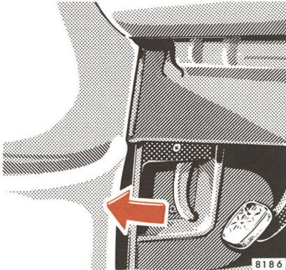
Pull lever below L-H side of instrument panel to unlock the hood. The hood opens to the safety catch stop. Pull lever in radiator grille as indicated by the arrow and lift hood (windshield wiper arms must not be folded out).
