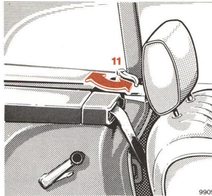
3. Insert both locking handles into the forward locks and swing outwards.
