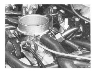
Remove air filter top cover and check whether exhaust gas is emitted from the recirculation line (arrow) in the throttle valve housing.
