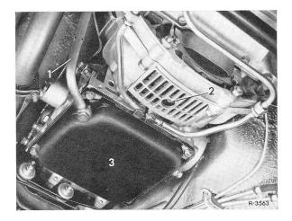
• Tighten fixing screws of oil pan with cork gasket (K 4 A 025 and K 4 B 050) to 8 Nm (0.8 kpm).
