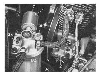
A Air suction intake and air release outlet 1 Air filter
